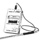
This is helpful when you want to check on the properfunctioning of the platinum resistance thermometer. e.g. if you suspect that it is not accurately controlling oven temperature.
